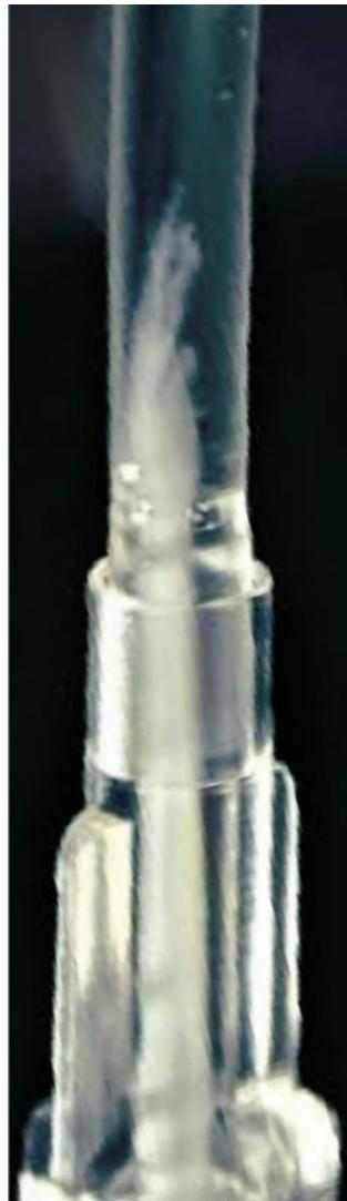
Fig. 1b: Physical precipitation of Midazolam as a result of an unfavorable pH medium [Riemann et al. 2005].
