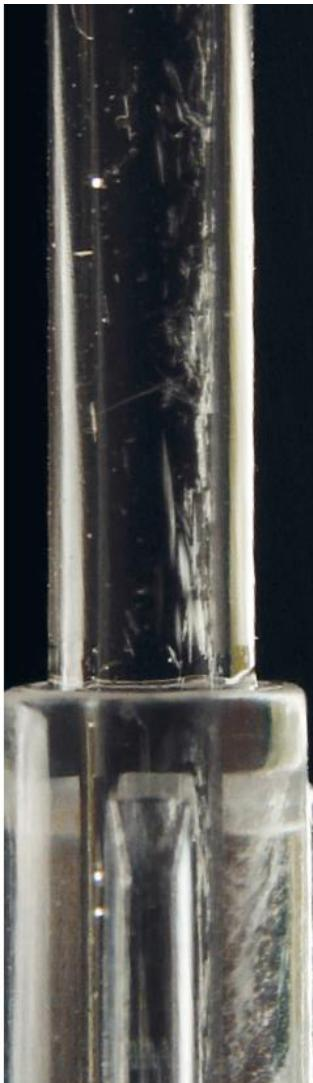
Fig. 1a: Chemical precipitation of Midazolam (turbidity) and Ketamin (particle formation) [Riemann et al. 2005].
